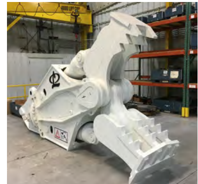
UPX 950 WITH CONCRETE PULVERIZER JAWS
