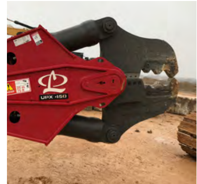
UPX 450 WITH CONCRETE CRACKING JAWS
