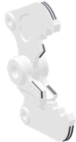
Cracker Wear Plate Location FIGURE 44
