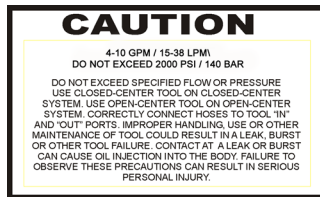
29188 GPM/Pressure Caution Sticker
