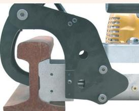
The DP3TH drilling machine is equipped with a four stroke petrol engine and is designed for drilling holes in rail for electrical connections and fish plates. This type of drilling machine features an over-rail clamping; so it is not necessary to remove the ballast but traffic has imperatively to be stopped during the drilling operation. This type of frame allows also drilling of the rail with counter-rail.
