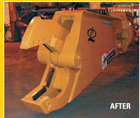
This 15 year old MSD shear, used heavily for scrap processing (above), was recently reconditioned to provide many additional years of service.
