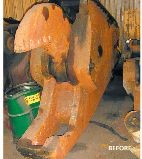
This 15 year old MSD shear, used heavily for scrap processing (above), was recently reconditioned to provide many additional years of service.
